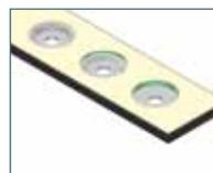
**THREE-LAYER BUS BAR UTILIZING EMBOSSED "DIMPLES" FOR COPLANAR INTERCONNECTION**
