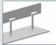
**SOLDER PIN CONNECTION WITH THERMAL RELIEF**
