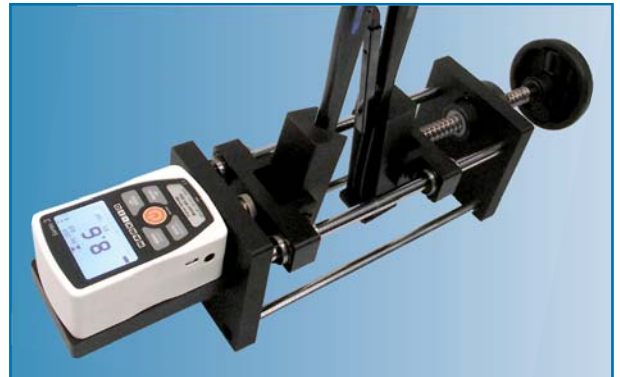
Handle force, measured at the factory, is a critical component of precise, reliable crimping.
